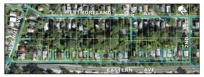
WSSC will install a new small diameter pressure sewer main in the roadway in front of homes. New pressurized sewer laterals will be installed around the sides of the homes to connect from the existing sewer exit point at the back of the home to the new main in the roadway. Each home will require a grinder pump to move wastewater from the basement level of the home (the existing sewer exit point) to the roadway at the front of the house.
