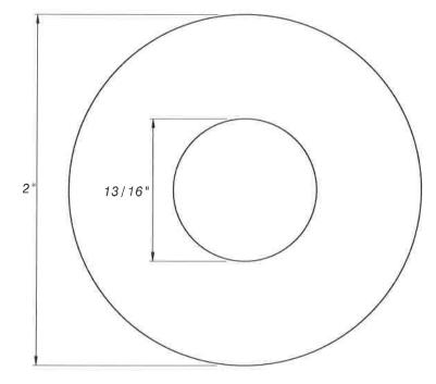
MATERIAL: LOW ALLOY STEEL IN ACCORDANCE WITH ASTM A307, LATEST REVISION THICKNESS:1/4"
