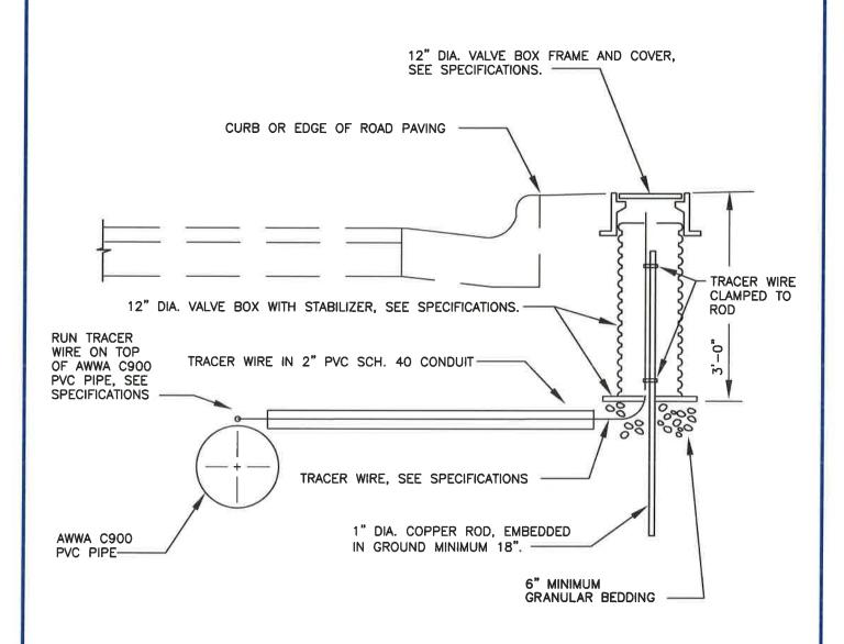
1. INSTALL TRACER WIRE IN 2" PVC SCH. 40 PVC WHEN NOT INSTALLED ON TOP OF PIPELINE.
