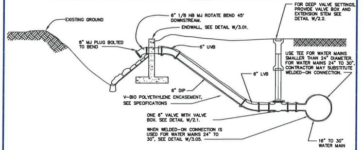
TYPICAL PROFILE FOR TYPE "B" BLOWOFF FOR MAINS 16" TO 30"
