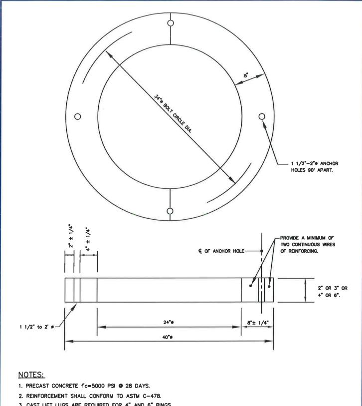
3. CAST LIFT LUGS ARE REQUIRED FOR 4" AND 6" RINGS.
