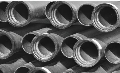
By switching to zinc-coated, V-Bio® encased ductile iron pipe, WSSC expects to put that pipe in the ground and not come back to replace it for 100 years or more.
