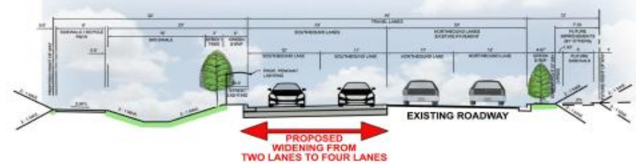
BRANDYWINE ROAD IMPROVEMENT TYPICAL ROAD SECTION SECTION 3
