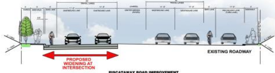
PISCATAWAY ROAD IMPROVEMENT TYPICAL ROAD SECTION SECTION 2
