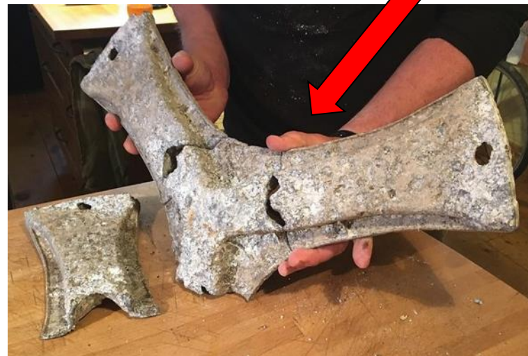
Corroded from Salt
