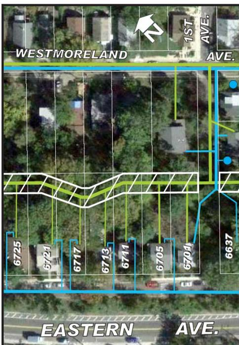
Note that a backyard alignment for all properties will require that the easements at addresses 6713 and 6717 Eastern Avenue extend deeper into the properties than the easements on neighboring properties. This alignment avoids installing a new sewer main across the existing gully at the rear of these properties.
