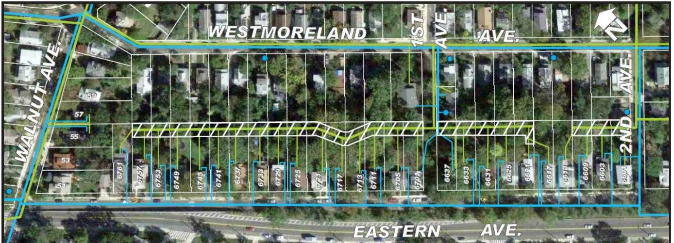
In the proposed backyard alignment solution, the gravity sewer mains for addresses 6703 through 6761 Eastern Avenue drain towards 1<sup>st</sup> Avenue.
