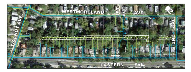
In the proposed backyard alignment solution, the gravity sewer mains for addresses 6701 through 6761 Eastern Avenue drain towards 1<sup>st</sup> Avenue. Affected properties are required to grant a 20-foot easement to WSSC at the rear of their properties. The property at 6621 Eastern Avenue must grant a larger easement to allow WSSC to connect to the existing sewer lateral at 6617 Eastern Avenue.
