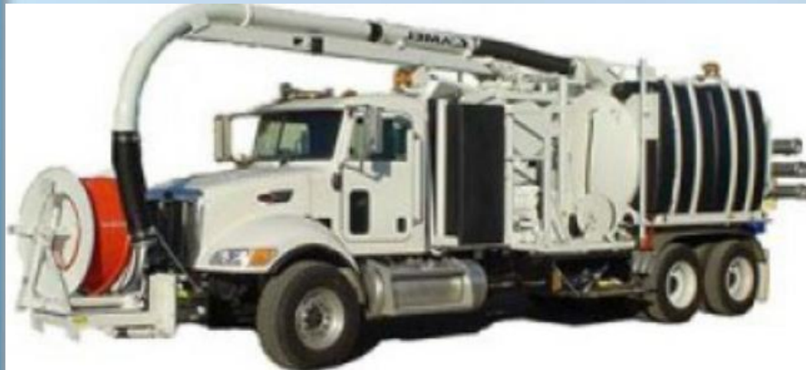
➤ Lining Jetting/Vacuum Truck
