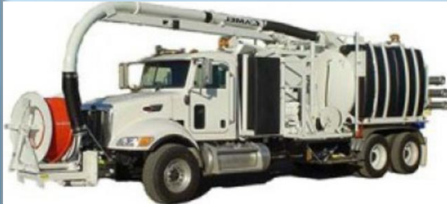
➤ Lining Jetting/Vacuum Truck
