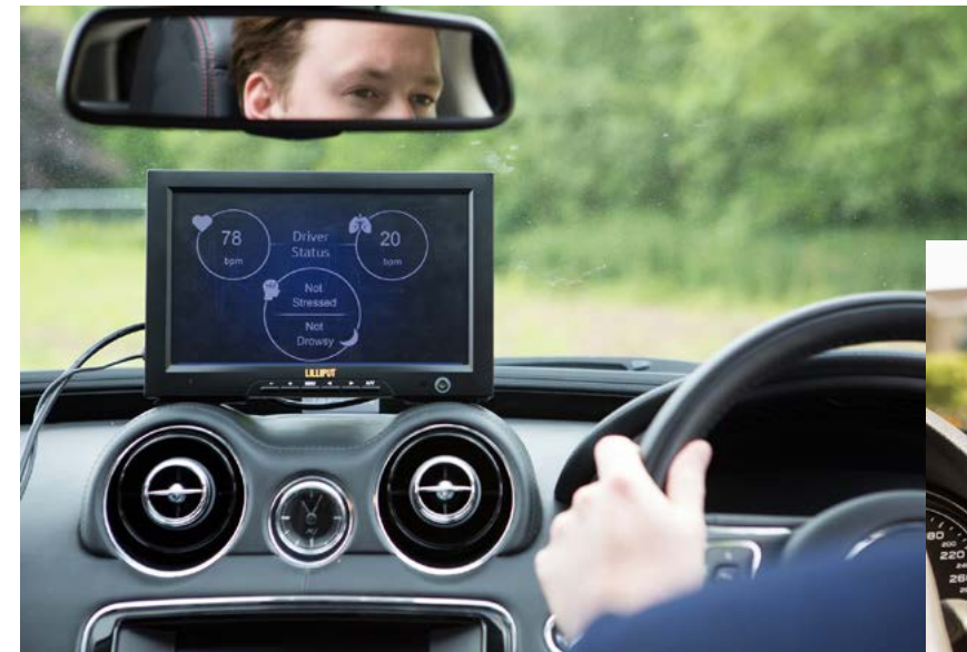
Jaguar Land Rover is testing ways to monitor well-being and concentration of drivers. Based on a technique used by NASA to improve concentration, sensors detect brainwaves through the hands via sensors embedded in the steering wheel to determine if the driver is focused, daydreaming, sleepy, or distracted.
