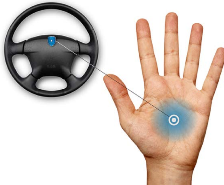
Sober Steering developed a touch-based alcohol interlock that is installed on the steering wheel. Upon ignition, a driver places a hand on the biosensor pad in the wheel, which detects alcohol by touch. If alcohol detected exceeds a pre-set limit, then the vehicle is immobilized and an instant message is sent to dispatch (or parents).
