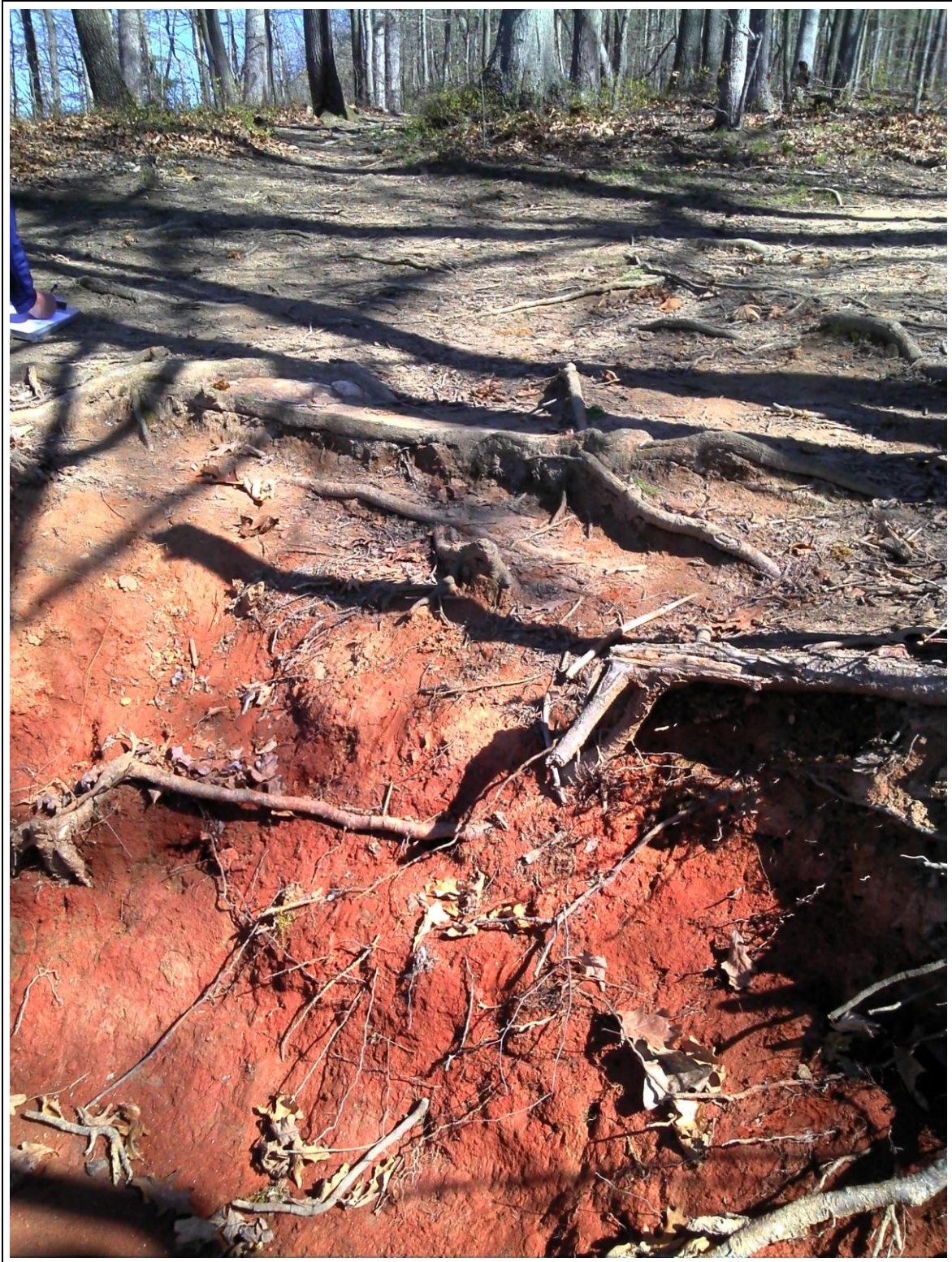
Photo 5-9: Brown's Bridge Recreation Area - North Bank shoreline collapsed area of red soil
