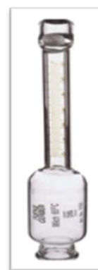
Figure 2.8. Standard Gerber Butyrometer Used for Milk Fat Determination (www.coleparmer.com)
