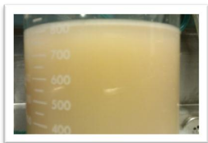
Figure 3.5. Wastewater from the Coffee Bar, Student Stamp Union, UMD, College Park, collected on 11/4/2010. (a) Sample at time of collection, (b) sample kept in the refrigerator at 4^{\circ}\text{C} for 14 days. Separation in form of suspended, floating, and settling clusters can be seen.
