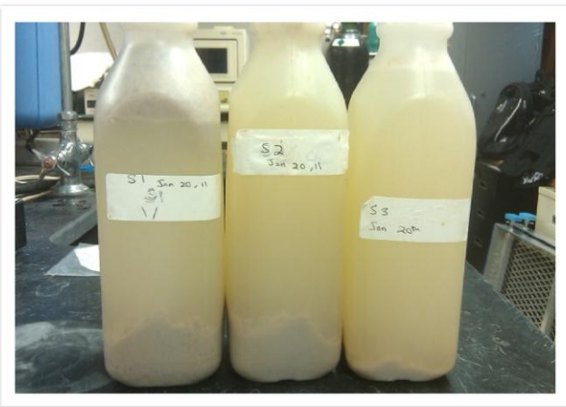
Figure 3.14. Specialty Coffee Shop Interceptor Samples Collected from Inlet (right), Middle (Center), and Outlet Compartments (Left) on 1/6 (a), and on 1/20 (b) Inlet (Left), Intermediate (Center), and Outlet (right)
