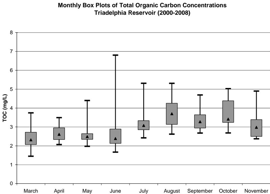
**Figure 39. Monthly Box Plots of TOC for Triadelphia Reservoir**
